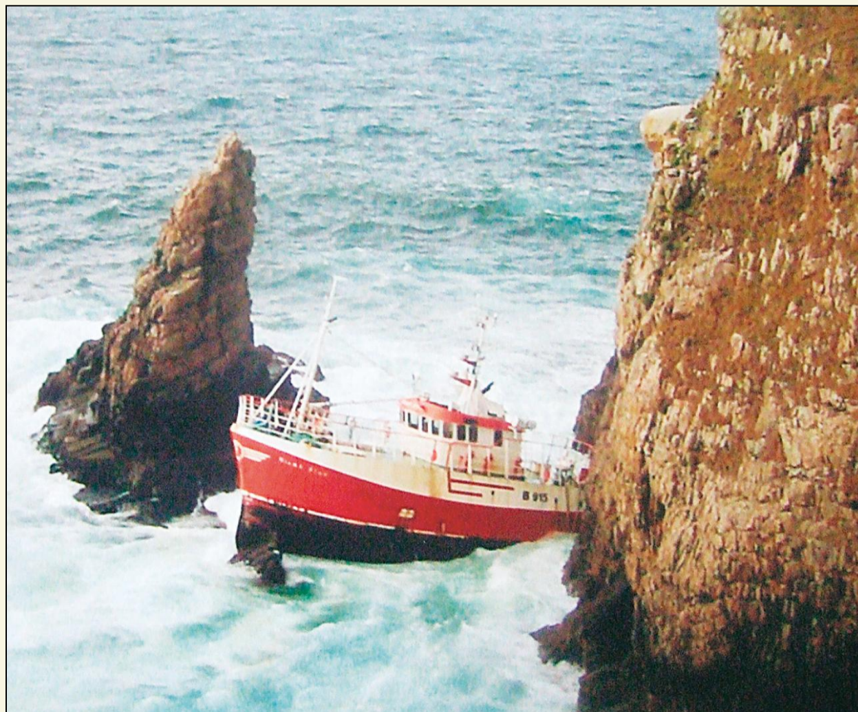
The Niamh Aine after running aground: the fishing vessel's master fell asleep in the wheelhouse
